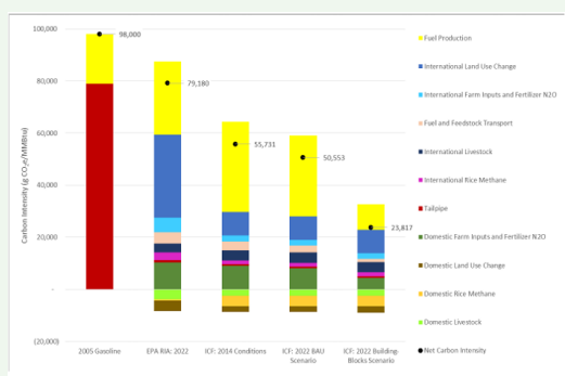
Figure 4. Full Life-Cycle Corn Ethanol GHG Results for the ICF: 2014 Current Conditions, ICF: 2022 BAU, and ICF: 2022 Building-Blocks Scenarios (Flugge et al., 2017)
